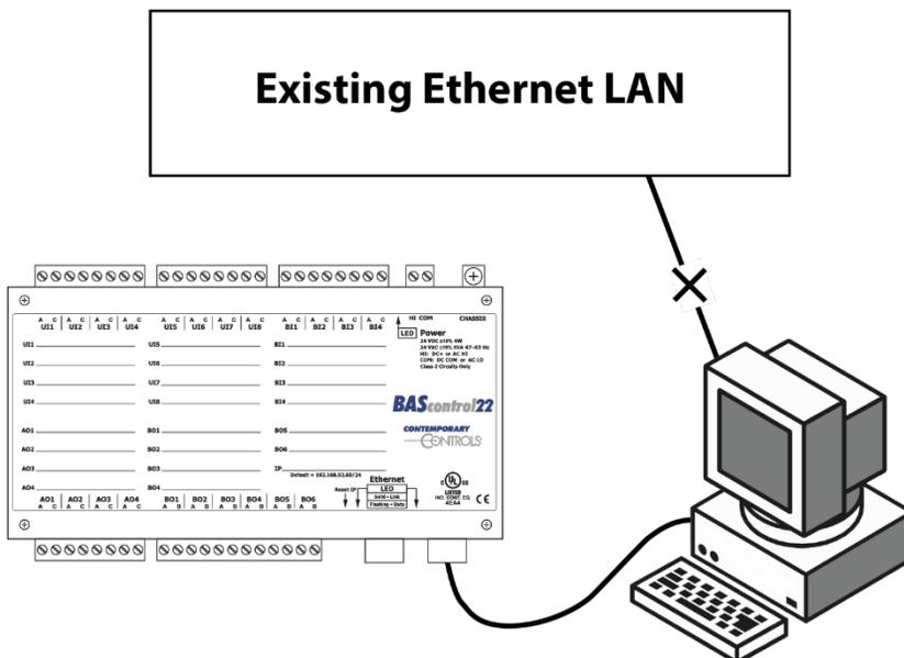
Figure 11 — Setup for Initial IP Address Configuration by Web Browser
