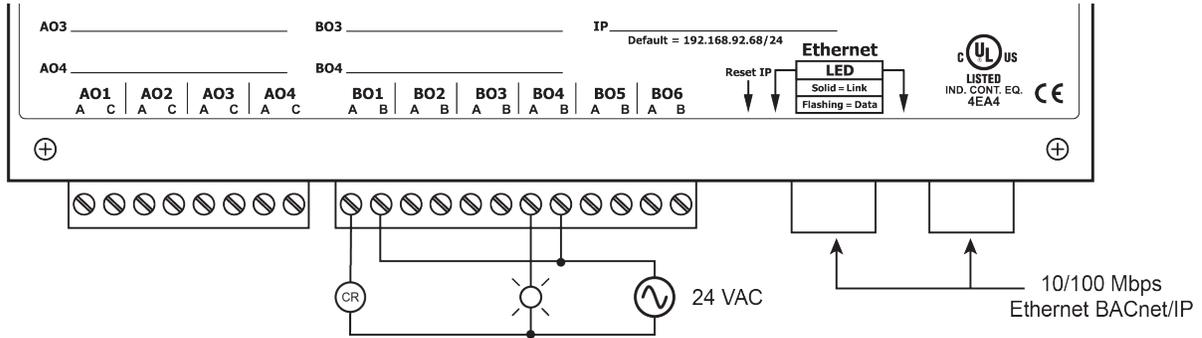
**Figure 9 — Binary Output Connections**
