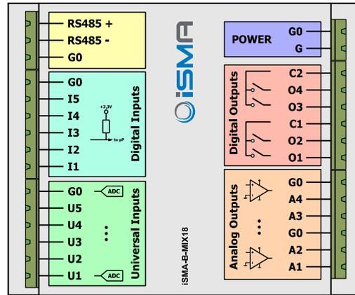
**All G0 terminals are connected together internally**
