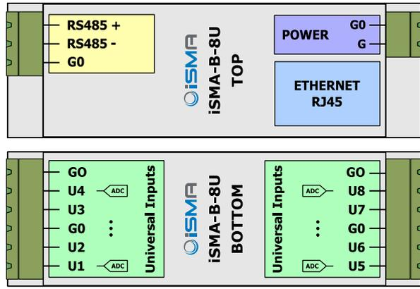
All G0 terminals are connected together internally
