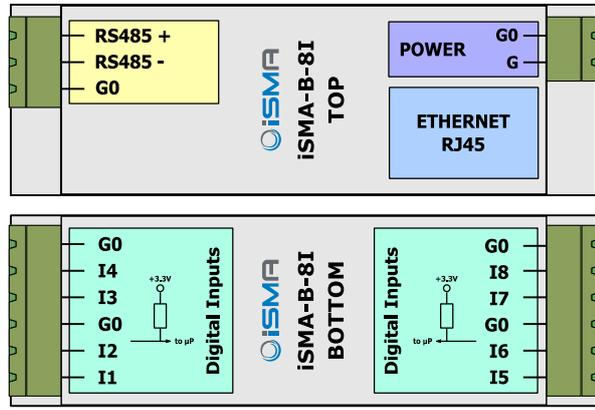
All G0 terminals are connected together internally
