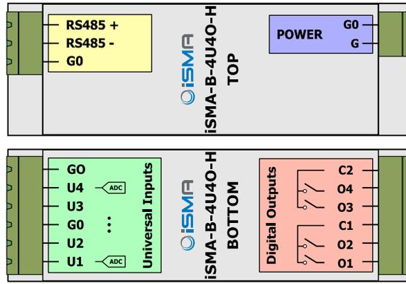
All G0 terminals are connected together internally
