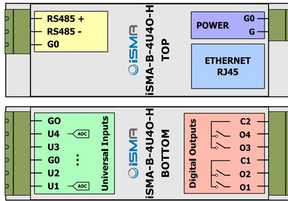
**All G0 terminals are connected together internally**
