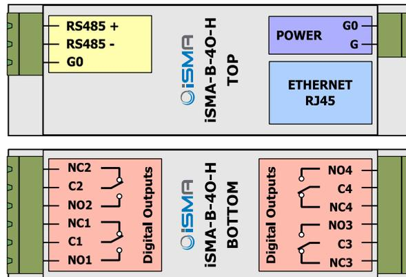
All G0 terminals are connected together internally
