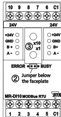
4. switch on the supply voltage of the module; it is now permanently saving the bit rate in an EEPROM;
