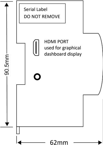
**NOTE:** Serial label covers the micro USB port which cannot be used to power the BASpi-Edge. Do not remove the serial label or BASpi-Edge warranty will be voided.
