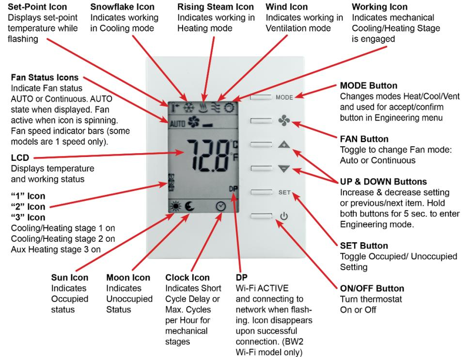
The BASstat has a built-in space temperature sensor with provision for remote wired 3kΩ NTC thermistor sensor, or temperature value can be sent by another device over the BACnet network.
