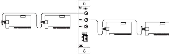
Figure 2 — A hub is required to extend bus segments.
