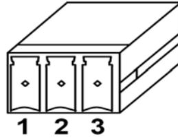
Figure 6 — Screw Terminal Connector Numbering Orientation
