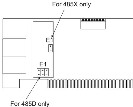
Figure 7 — Jumper settings for EIA-485 models.
